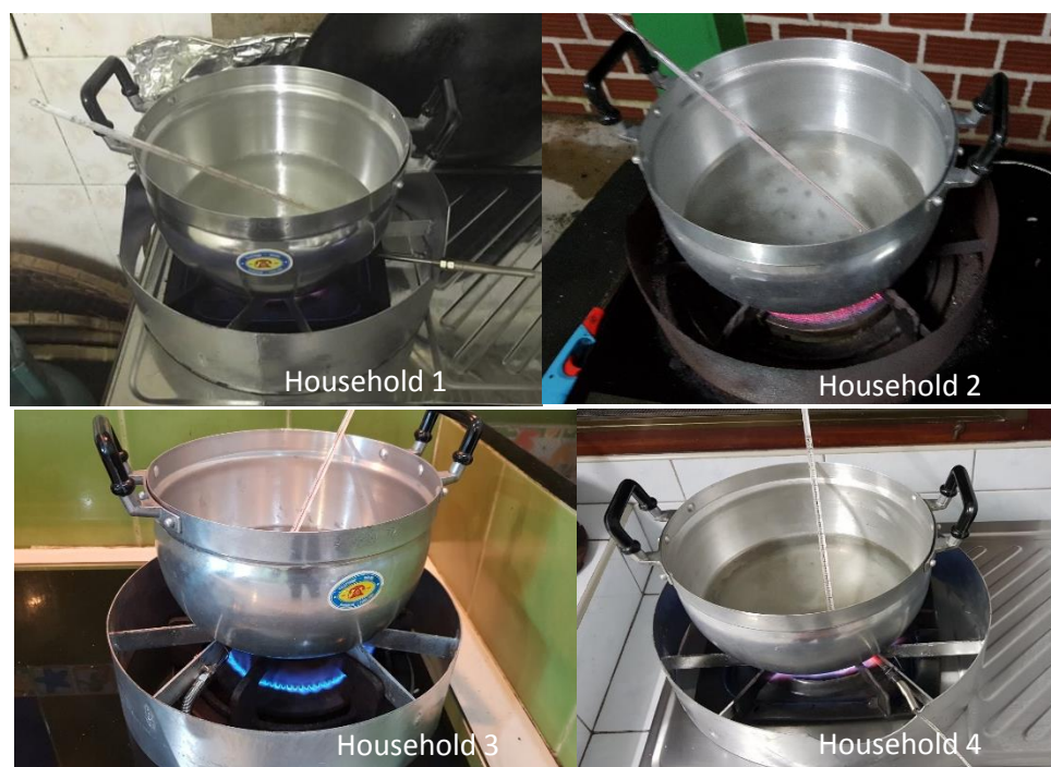
Figure 3. The LPG cooking stove of thermal performance testing
