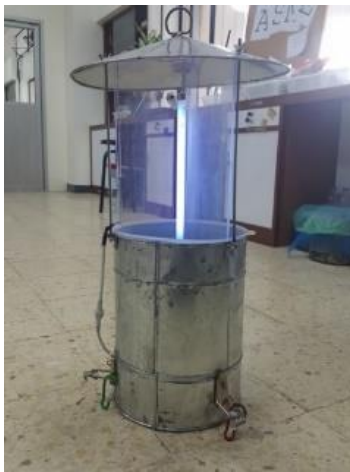
Figure 2. Pennsylvania light traps with Philips TL 8W actinic BL light bulb
